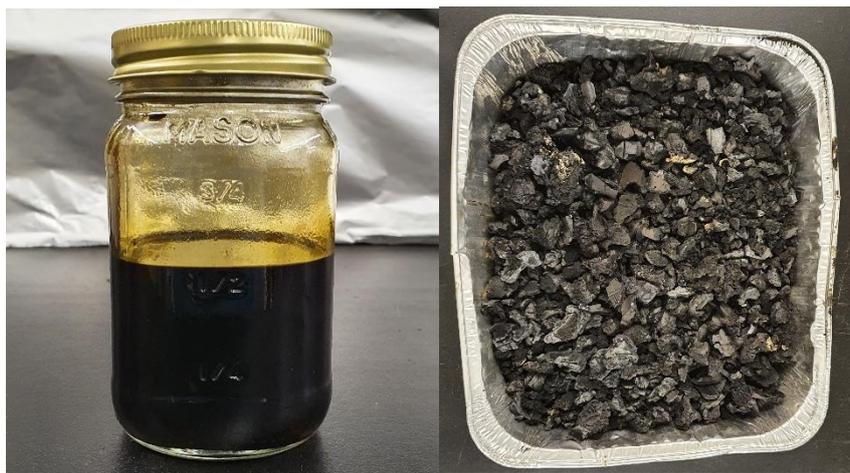
Figure 18 - Oil and char from rubber pyrolysis
