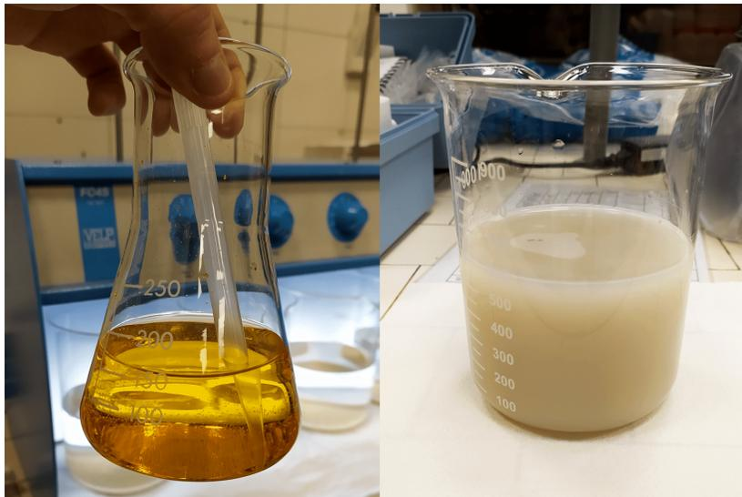
Figure 4.2: 1:50 dilution ratio of Drewo8016<sup>®</sup> with demineralized water (left) and freshly prepared bentonite suspension (right)
