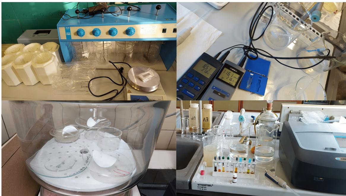
Figure 4.1: Jar test apparatus, portable turbidimeter, beakers and magnetic stirrer (upper left), portable turbidimeter and pH-meter and quartz cuvettes (upper right), desiccator and membrane filters (lower left), cuvet kit tests for chemical analyses, adjustable micropipette, vacuum pump glass chamber and spectrophotometer DR6000 (lower right)
