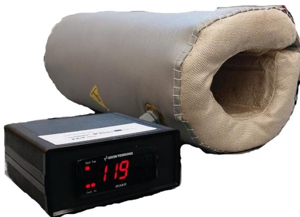
Figure 14 Electric heater and electronic thermo controller.
