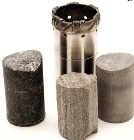
Figure 1 Baker Hughes MaxCOR large-diameter rotary sidewall plugs (McPhee et.al., 2015).
