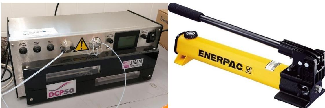
Figure 13 High precision pump (left) and manual hydraulic pump (right)
