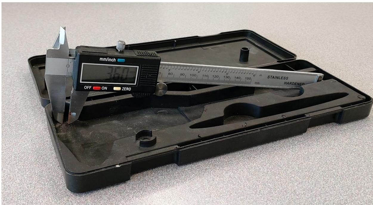
Figure 8 Digital caliper
