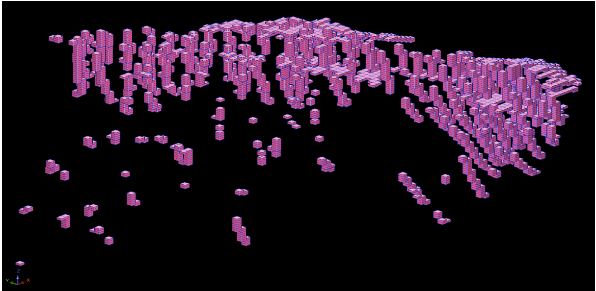
Figure 5.3(a): Display of constrained block model Block Model Sub-celling of a block mode in surpac
