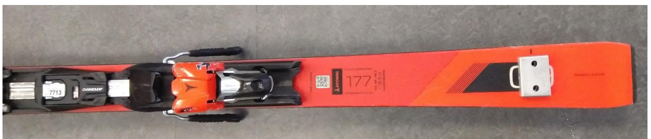
Figure 9: Aluminum case placed on the rear part of the ski to allocate the sensor.
