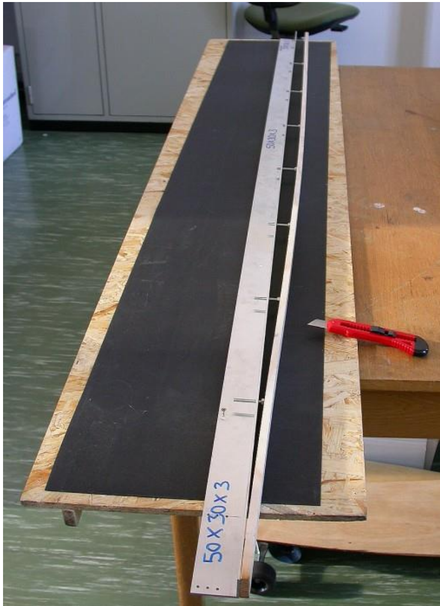
Figure 3: Layer of UHMW-PE ready to be shaped for ski construction. Picture from [9].
