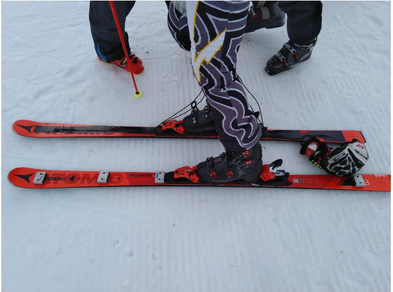
Figure 11: Disposition of the accelerometers' measurement system (in foreground). On the right ski is mounted another measurement system involving piezoelectric sensors for other purposes and not relevant for this study.
