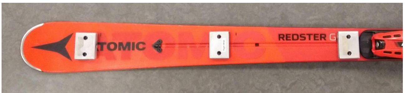
Figure 8: Aluminum cases placed on the front part of the ski to allocate the sensors.
