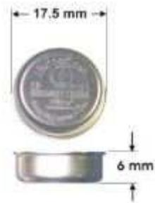
Figura 5.6: Sensori wireless I-button Maxim Integrated DS1923
