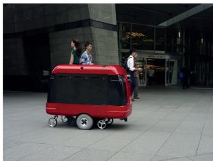
CarriRo® Deli, which was developed with the aim of realizing the world's first delivery robot service, is a delivery robot that uses Autonomous Driving technology equipped with a loadable box.
