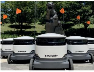
The project was established in 2014 and runs on the sidewalk. Pilot distribution began in 2016. It has multi-sensor fusion technology, based on LIDAR, machine vision, depth senor, etc., has the ability to locate and navigate high precisely indoors
