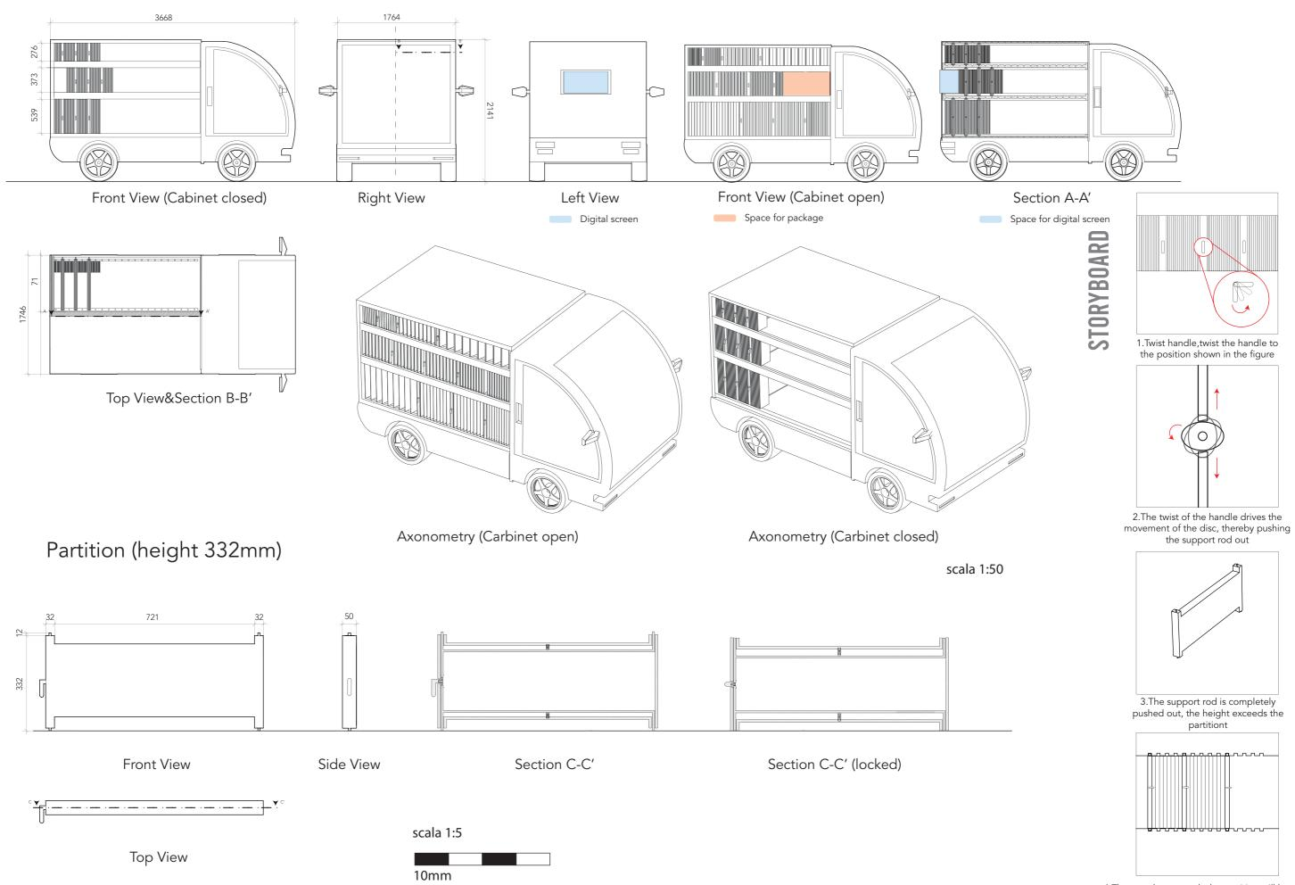
4.The part that exceeds the partition will be stuck in the card slot to fix the position of the partition
