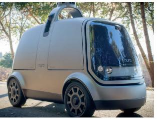
Nuro solve problem of local commerce with last-mile delivery of consumer products, groceries, and hot food from local stores and restaurants. With its specially designed size, weight, pedestrian-protecting front end, operating speed, electric propulsion, and cautious driving habits.
