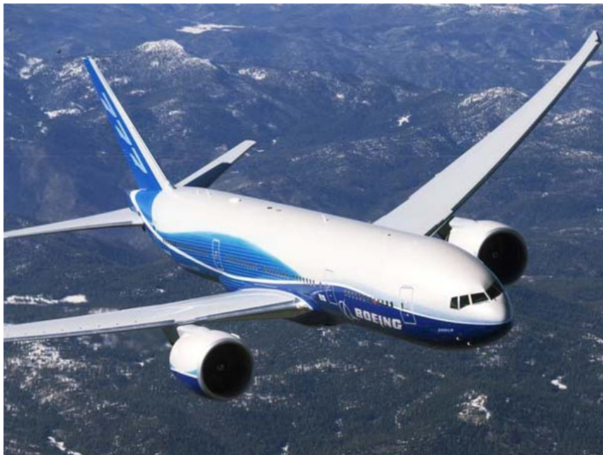
Figure 2.16: The B-777 Airframe Incorporates Durable Lightweight Composite Aircraft Structures, Including Graphite Epoxy Floor Beams, Flaps and Tail Assembly
