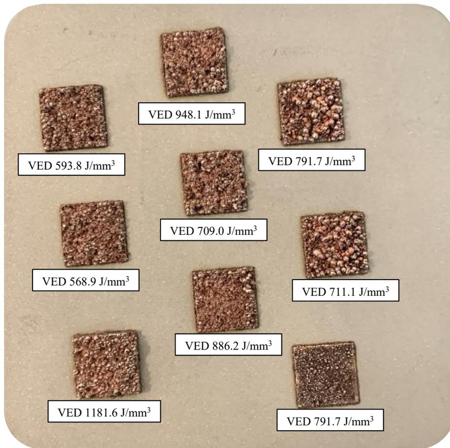
Figure 66 – Job 4. Cu – 0.5 wt.% milled C
