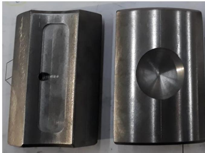
**Figure 37.** Small bearing pads.
