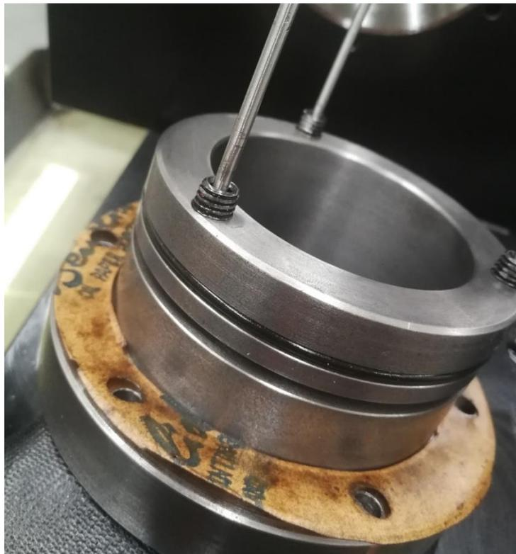
**Figure 42.** Pipes and stopper preassembly.
