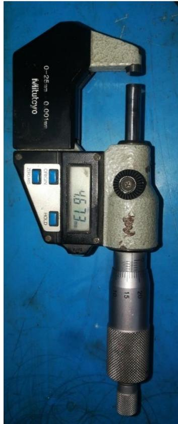
**Figure 32.** Digital feeler gauger with millesimal resolution used to calculate the plate arrow.
