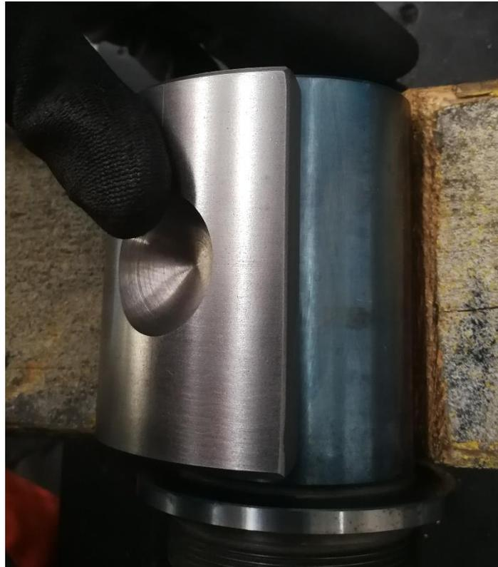
**Figure 70.** Step 1 – Putting the bushing on the engineering blue on the spindle.
