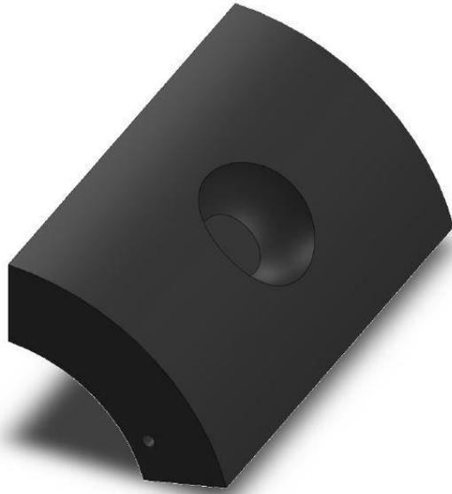
**Figure 19.** External side of the bigger bearing pad.
