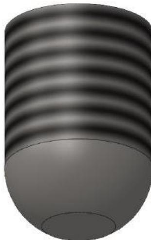
**Figure 17.** Support of hydrostatic bearing pad.
