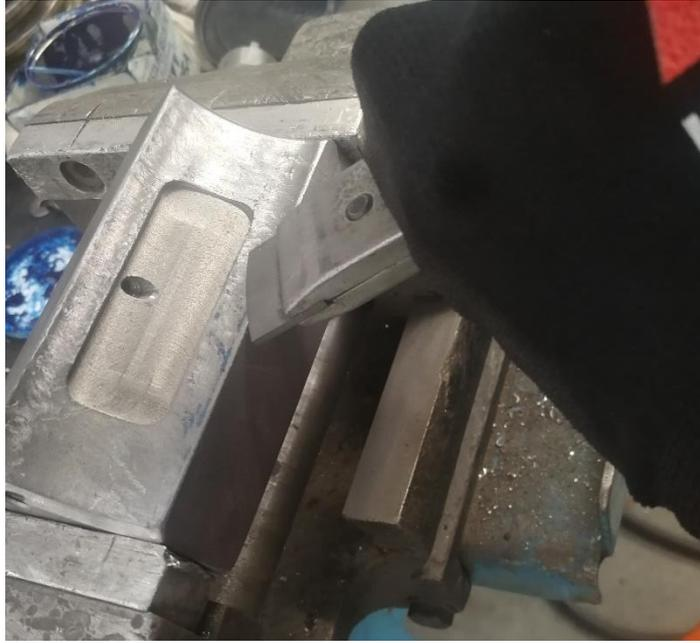
**Figure 72.** Step 3 - Scraping process.
