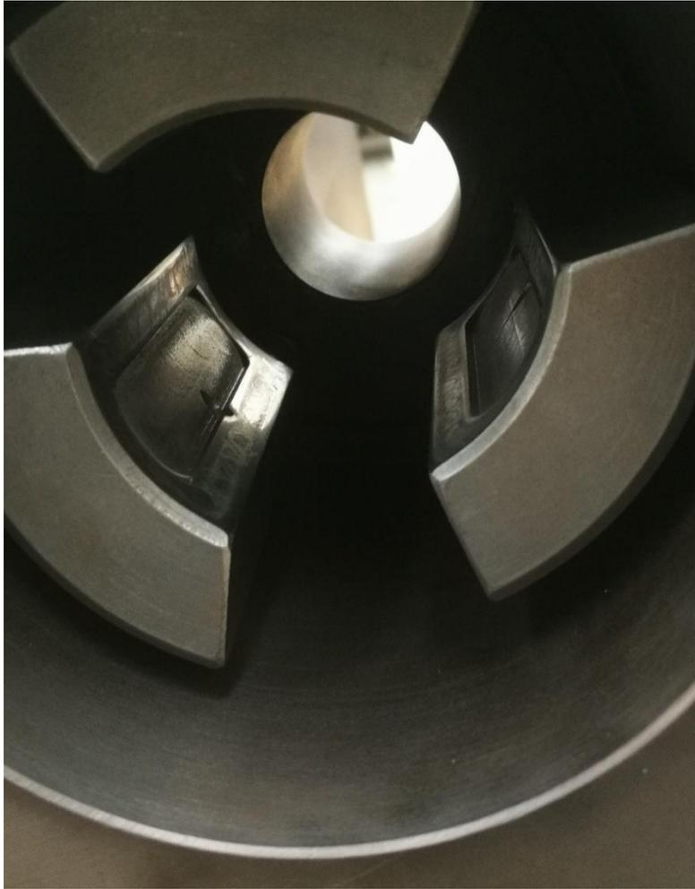
**Figure 45.** Bushings assembled inside the case.
