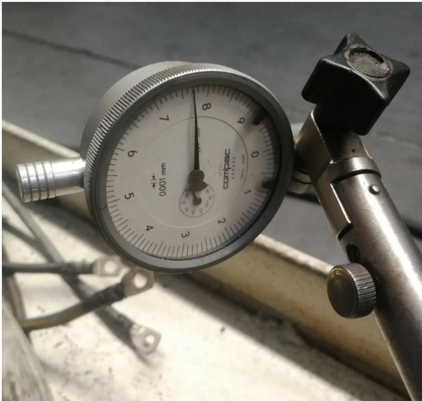
**Figure 36.** *Micrometric dial indicator device.*
