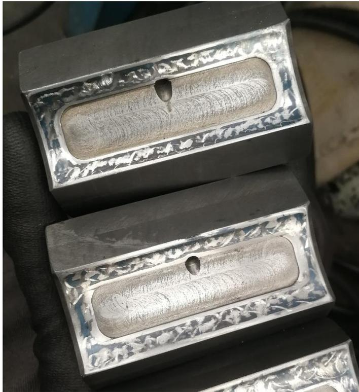
**Figure 73.** Final result of scraped pads.
