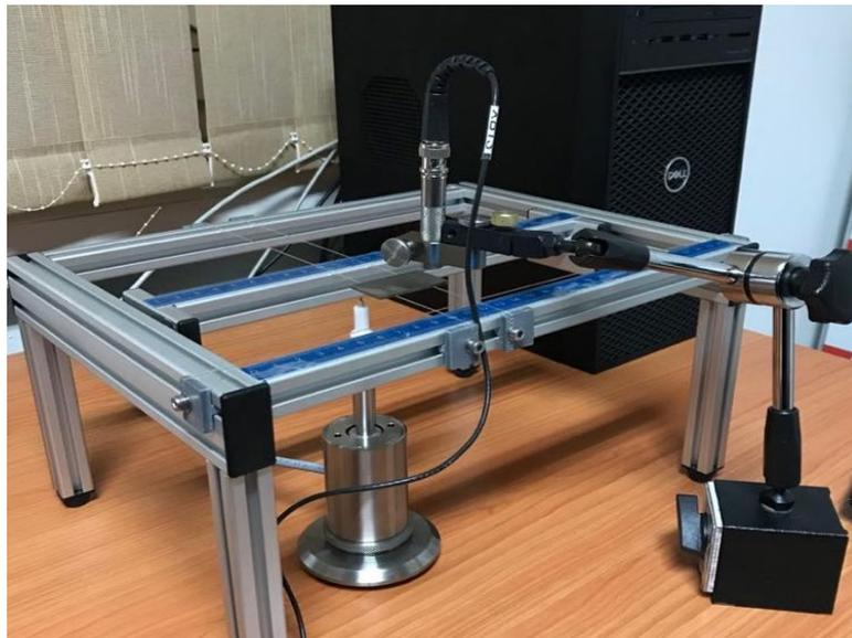
*Figure 53: Set-up for dynamic Young's modulus, dynamic shear modulus and Poisson's ratio at room temperature*
