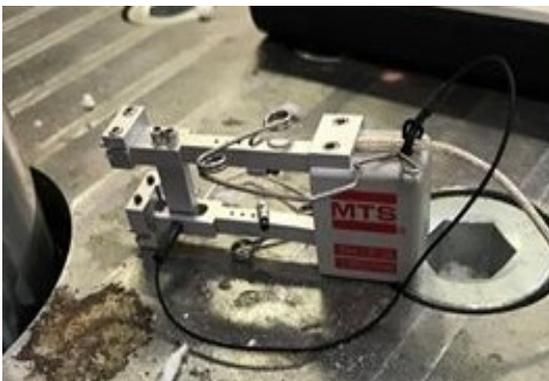
Figure 27: Axial extensometers MTS 634.12F-25
