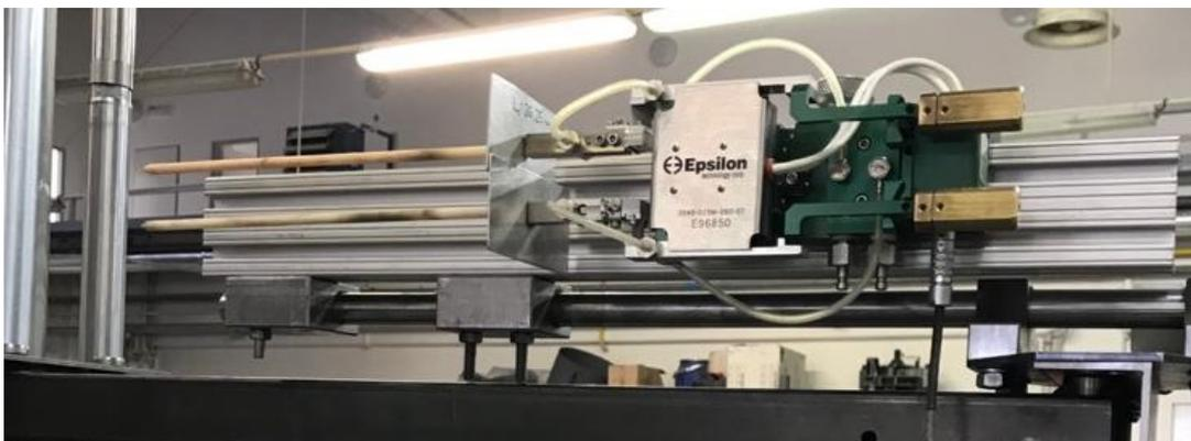
Figure 29: Axial extensometer Epsilon model 3549
