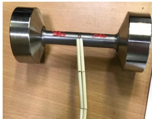
Figure 32: thermocouple welded to the specimen
