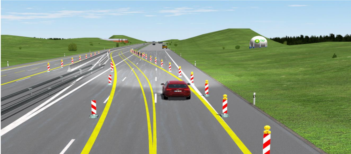
Figure 32 – Work in progress traffic signals
