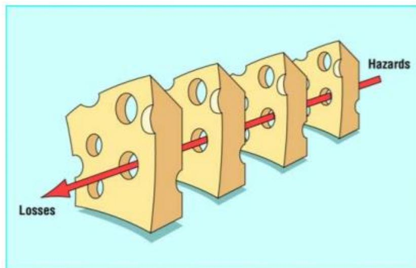
Figure 5-1 Representation of the hazard-barrier-error bond (Swiss cheese).
