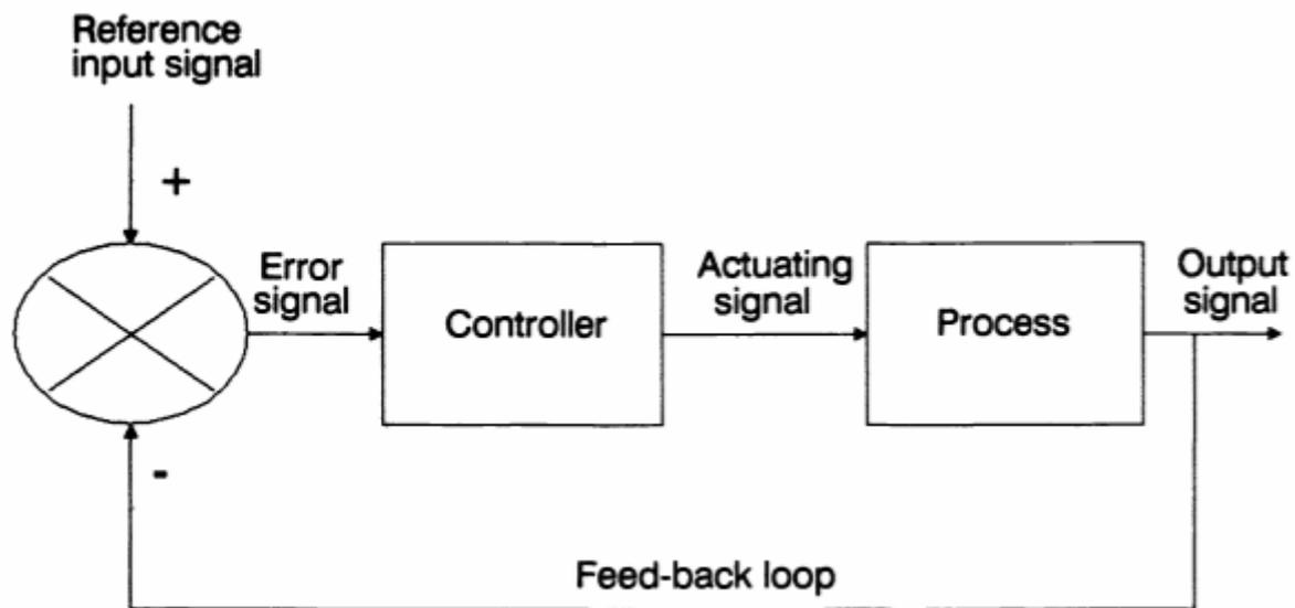
Figure 4-6 Basic feed-back loop: the difference between the output and input signals.
