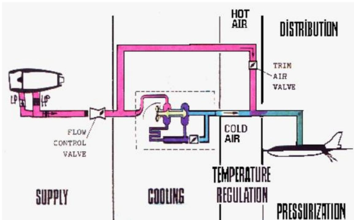
Figure 2-7 Air cooling system schema.
