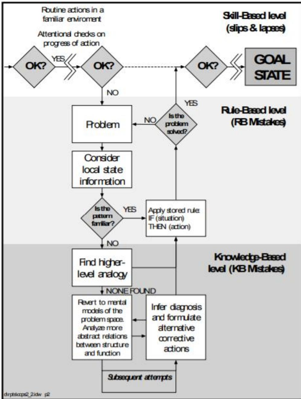
Figure 4-4 Dynamics of Generic Error Modelling System (GEMS)
