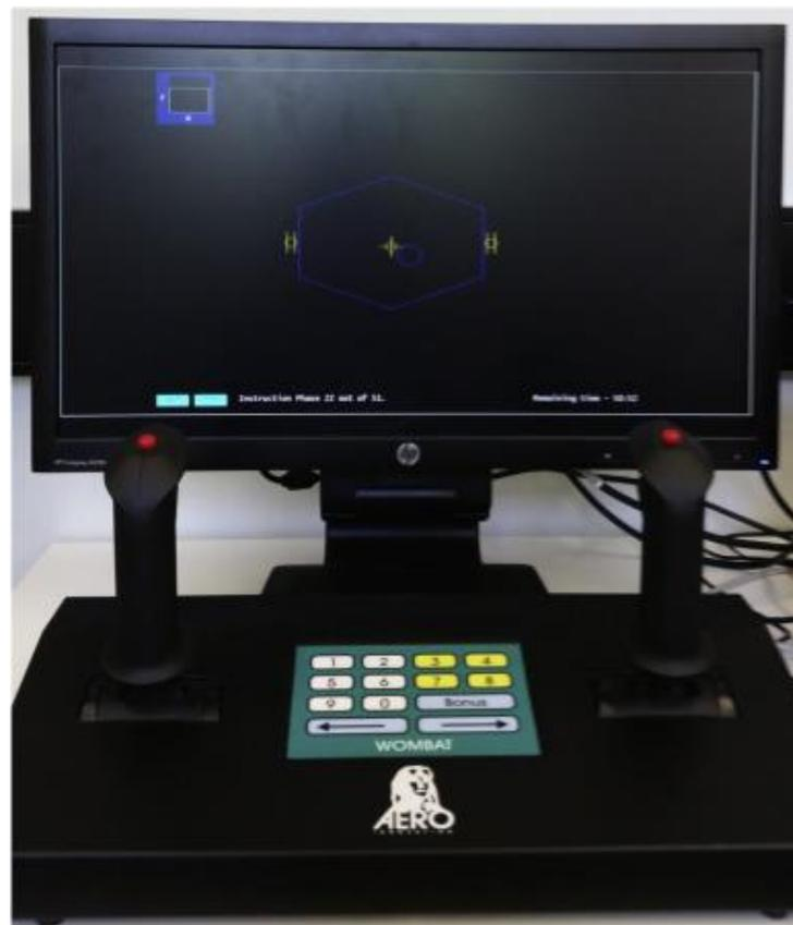
Figure 3-3 WOMBAT console with dual joysticks, keypad and tracking task on screen.
