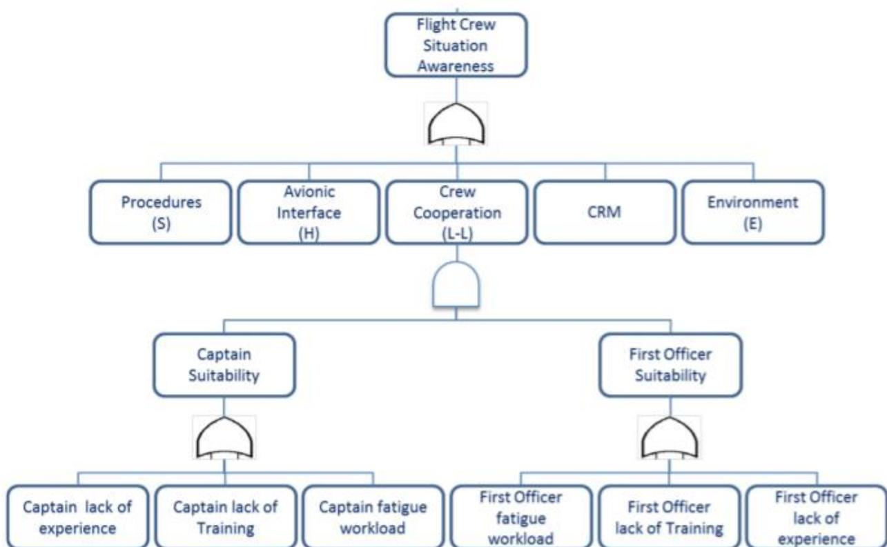
Figure 1-3 Fault Tree model of HF of FCSA.
