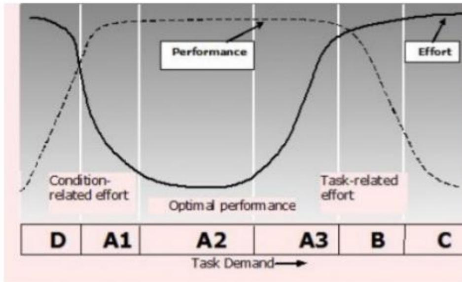
Figure 2-1 Relationship between workload and performance: six theoretical levels (de Waard,1996).
