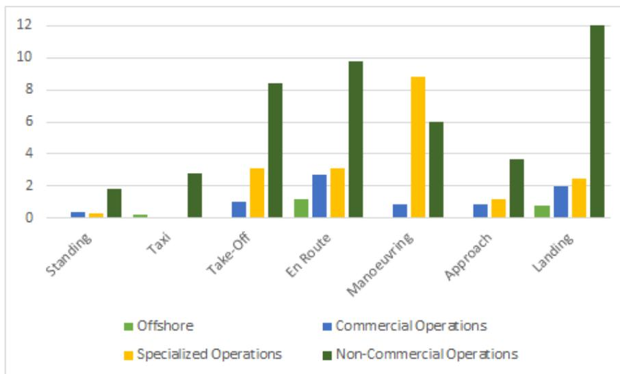
Fig 1.3.2: 2008-2018 Helicopter accidents and serious incidents by phase of flight - Source: EASA
