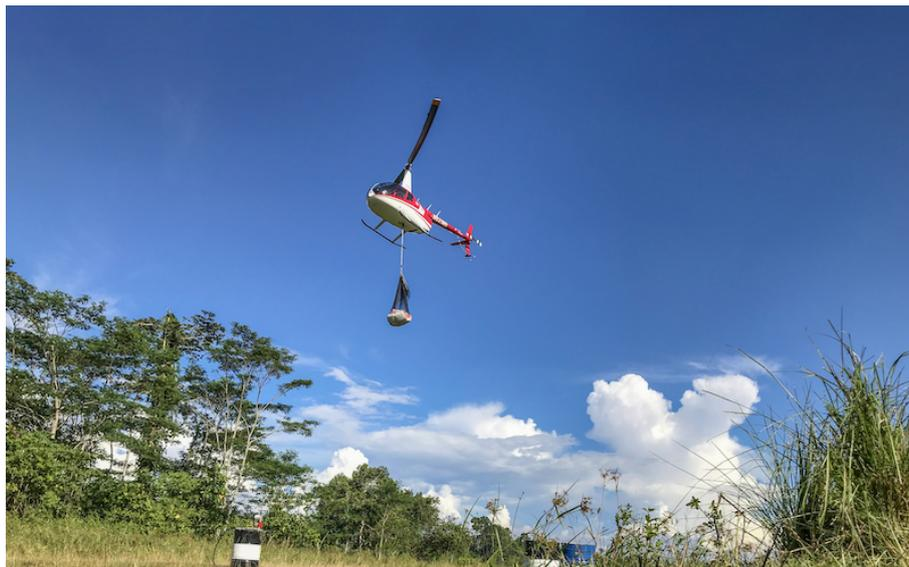
*Fig 1.2.1: Sling load transport operation*
