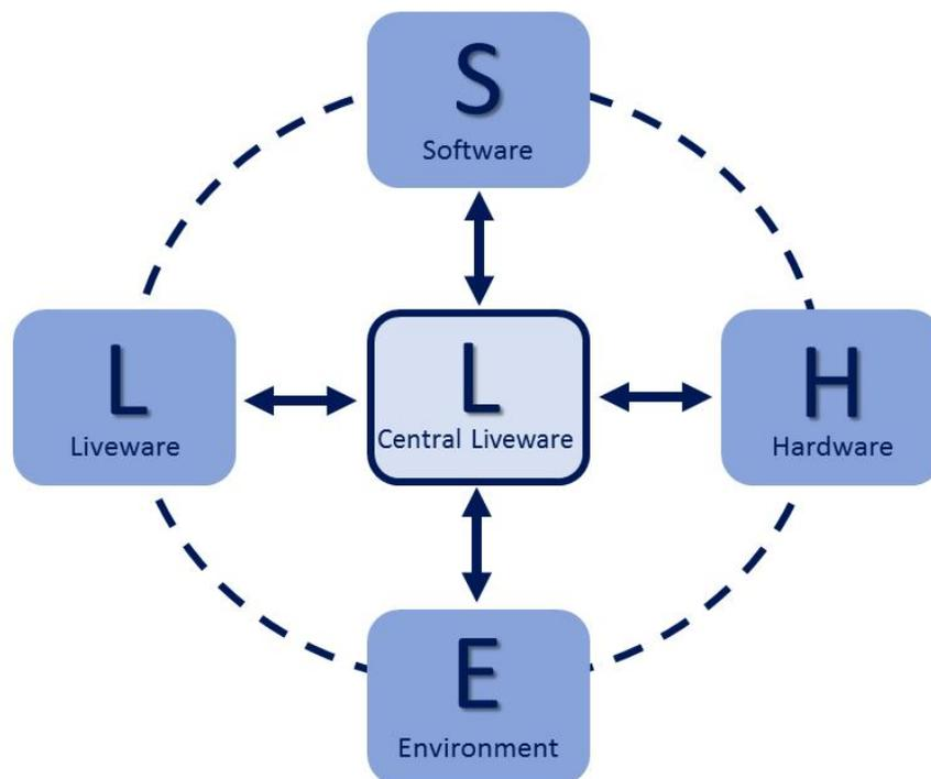
Fig 2.2: SHELL Model graphical representation
