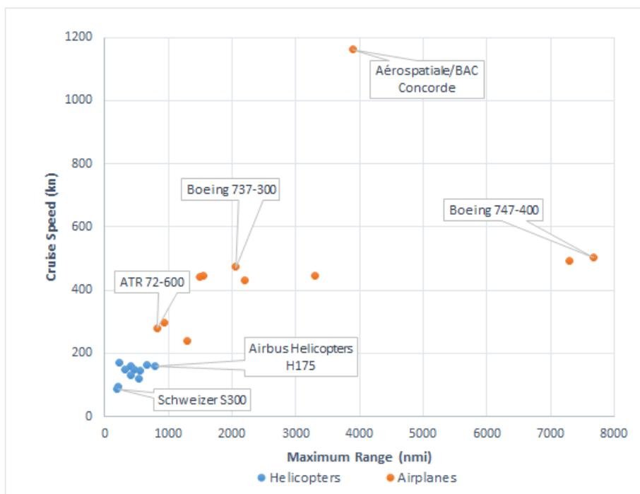
Fig 1.1.4: Maximum Range - Cruise Speed Diagram
