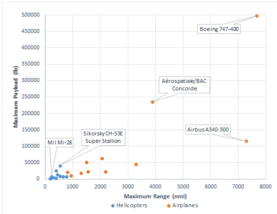
Fig 1.1.3: Maximum Range - Maximum Payload Diagram
