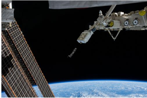
Figure 1.7: CubeSat deploy from NRCSD at tip of JEMRMS [22].
