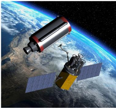
(a) A chaser spacecraft approaching a tumbling rocket body debris target using a gripper arm [40].
