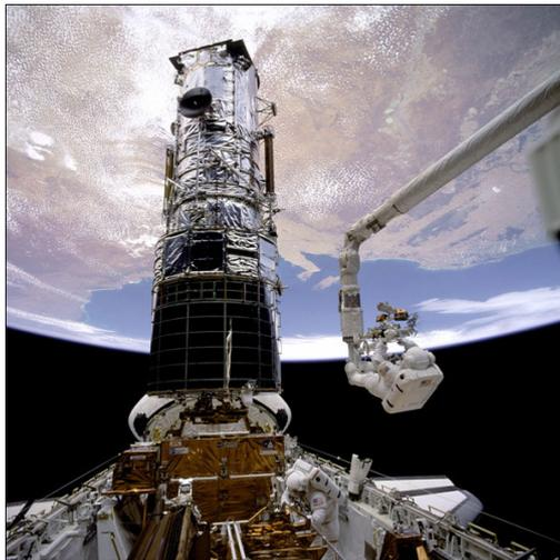
Figure 1.4: An astronaut anchored to the end of the Canadarm is being lifted up to the top of the Hubble telescope to install protective covers on the satellite [15].
