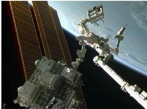
Figure 1.6: The Robotic Refueling Mission (RRM) investigation uses the International Space Station's Canadarm2 and the Canadian Dextre robot (right) to demonstrate satellite-servicing tasks [20].
