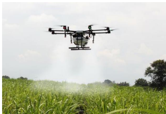
Figure 1.7 Multirotor UAV performing a spraying mission [5]
