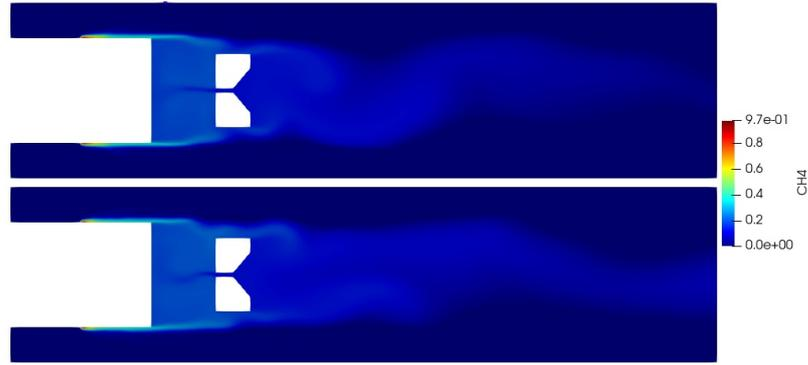
**Figure 4.11:**  $CH_4$  distribution for  $U_a = 50 \text{ m/s}$  (top) and  $U = 100 \text{ m/s}$  (bottom)
