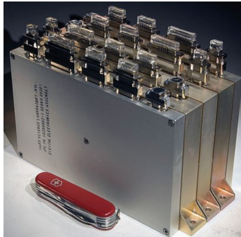
Figure 3.21: DEA package for MAHLI, Mastcams and MARDI: each instrument is a separated unit [33].
