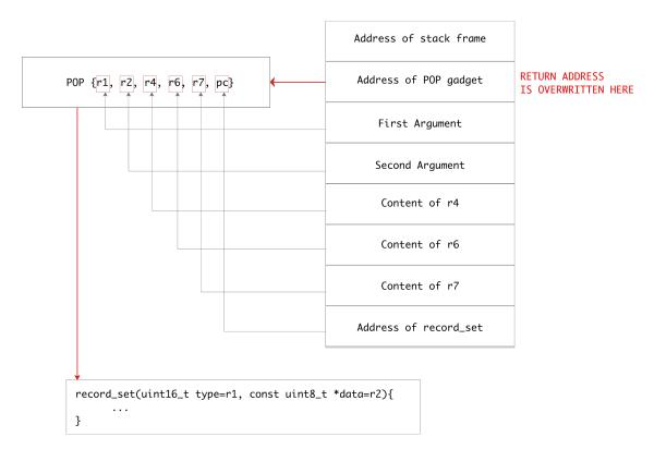
Figure 4.5. Layout of the ROP chain. Red Arrows show the flow of execution of instructions. From the POP instruction, the registers are loaded and control flow is transferred to the record\_set function
