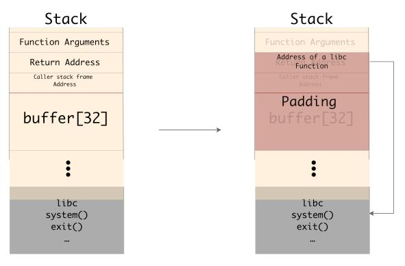
Figure 2.2. Exploitation of a buffer overflow for a return-to-libc attack
