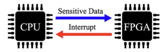
Figure 4.1. Simple communication schema between CPU and FPGA, taken from [24]
