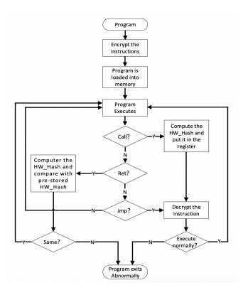
Figure 2.12. General schema of Branch protection through encryption
