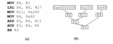
Figure 3.1. Code Snippet and origin tree of the R3 register
