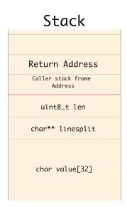
Figure 4.4. This is the layout of the stack when entering the readChar function. The buffer value is 32 bytes long and before the stack base there are two other variables.
