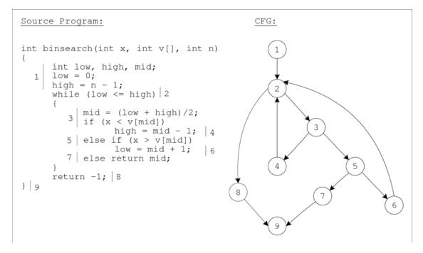
Figure 2.6. Example of Control Flow Graph
