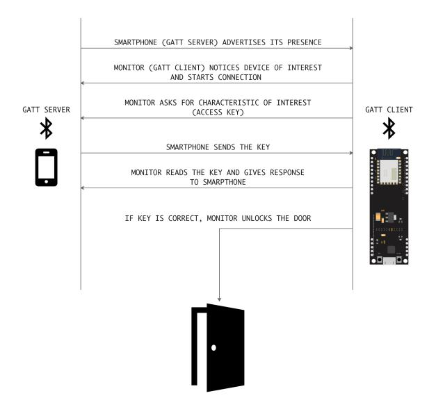
Figure 4.2. Here the architecture of the monitoring system, as well as the exchange of data between the two main parts, is schematized
