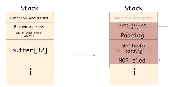
Figure 2.1. Stack before and after code injection. The return address is overwritten with the address of the injected code
