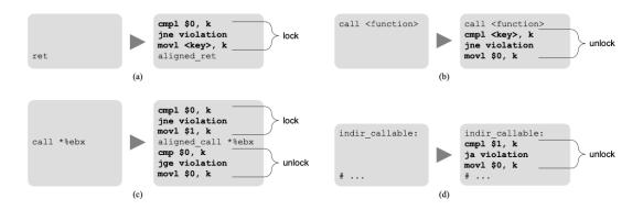
Figure 2.8. Code Instrumentation proposed in [3] in the different typologies of control transfer sites.
