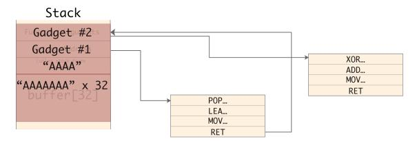
Figure 2.5. Stack's situation after ROP
