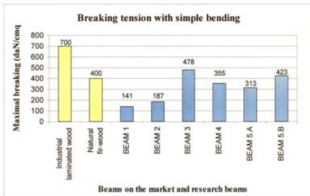
Breaking tensions obtained in laboratory tests reached great results, particularly for beams realised with melamminic glue which reached a breaking as good as heart-wood's one. The beam made disposing laminae vertically even exceeded natural fir-wood's breaking tension. All beams have regular deformations (arrows and lengthenings/shortenings of the centre-line section) both when adding load and when taking it away.
