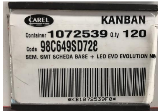
Figure 2.9. Internal electronic Kanban in Carel production lines.
