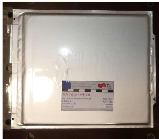
*Figure 2.1 - Pouch cell employed in tests*
