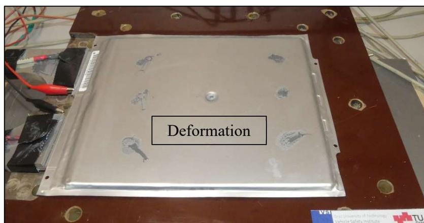
*Figure 2.6 - Cell after mechanical deformation*
