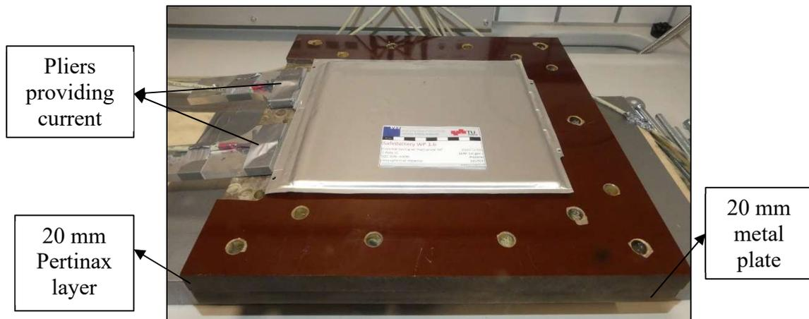
Figure 2.4 - Test bench set up with lower insulating layer
