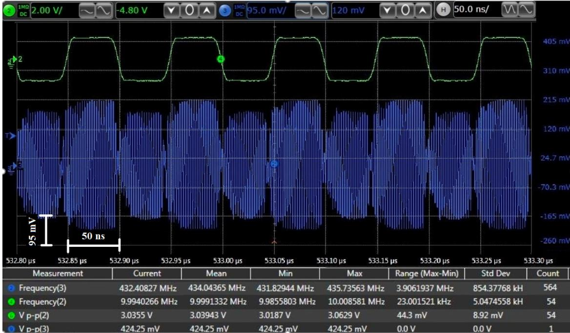
Figure 6.2: Measurement of the RF ASK transmitter.
