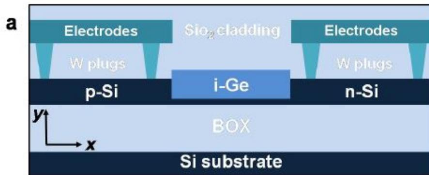
Figure 1.31: Cross-sectional schematics of a waveguide-integrated photodetector with a lateral silicon-germanium-silicon hetero-junction. [5]
