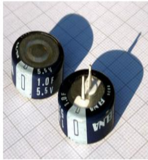
Radial style of a supercapacitor for PCB mounting used for industrial applications
