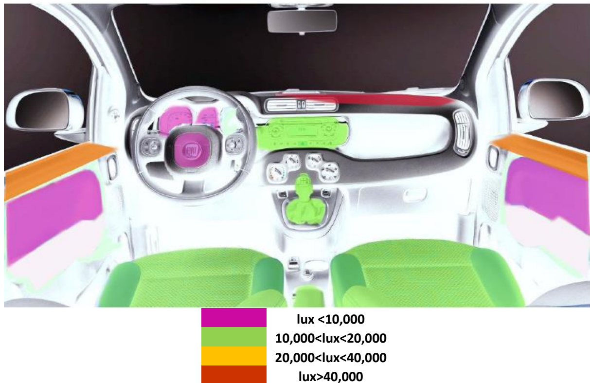
Figure A.1. Demonstration of interior illuminance of segment A by colors
