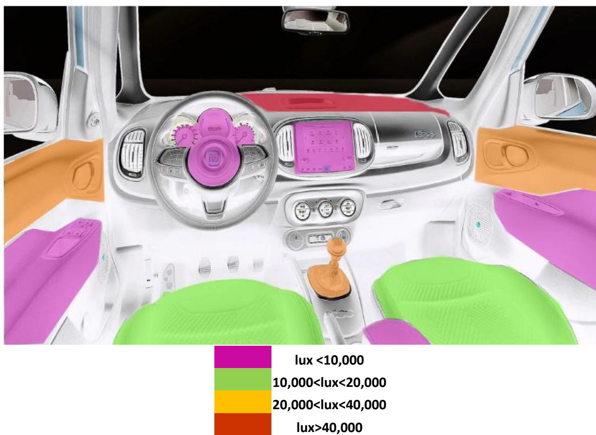
Figure A.3. Demonstration of interior illuminance of segment B by colors
