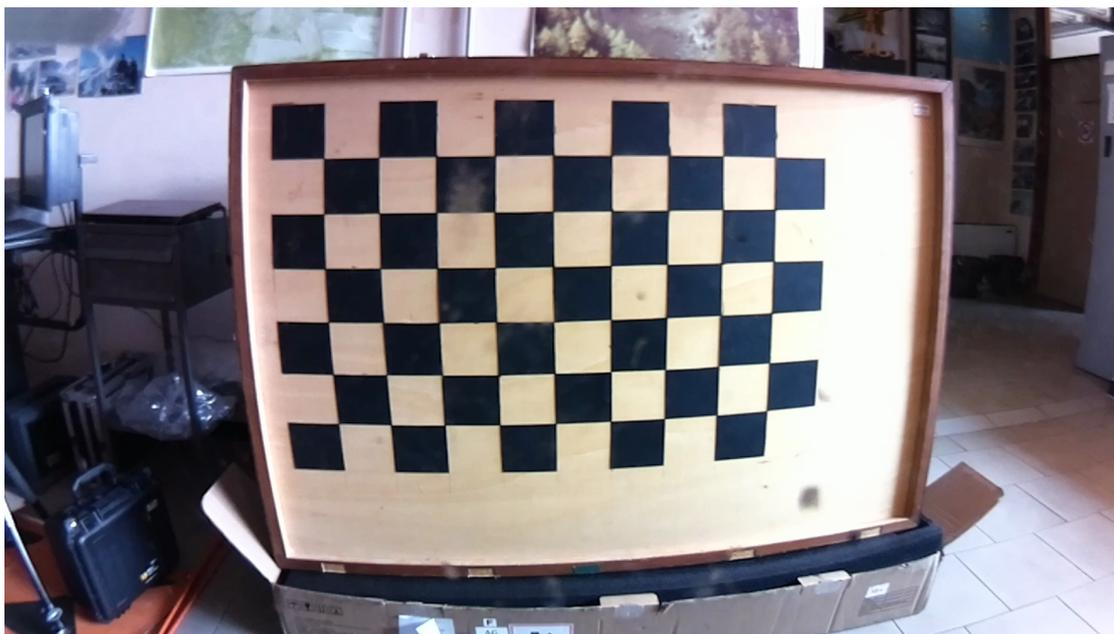
**Figure 4.2:** Chessboard used for the camera's calibration
