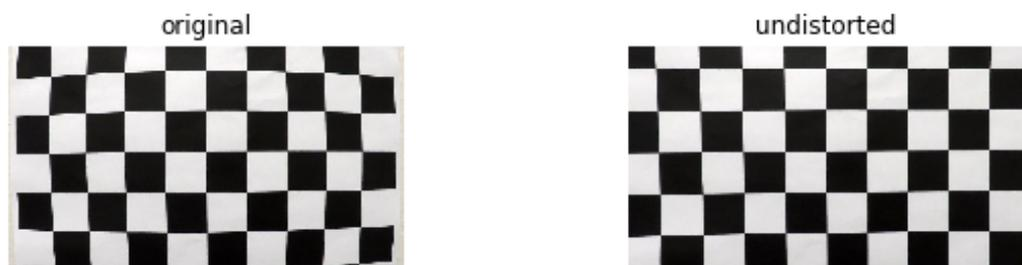
**Figure 4.1:** Effect of the distortion correction
