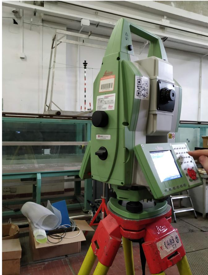
**Figure 5.21:** Tracking the movement of the platform with the total station
