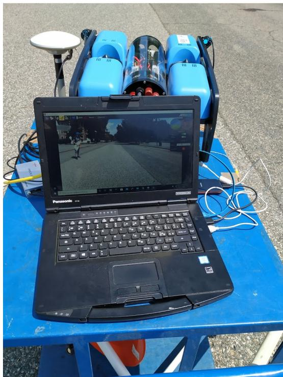
**Figure 5.10:** BlueROV2 with GPS antenna
