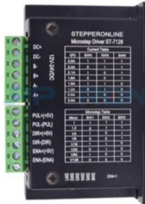
Fig.27 – Bipolar Stepper Motor Driver
