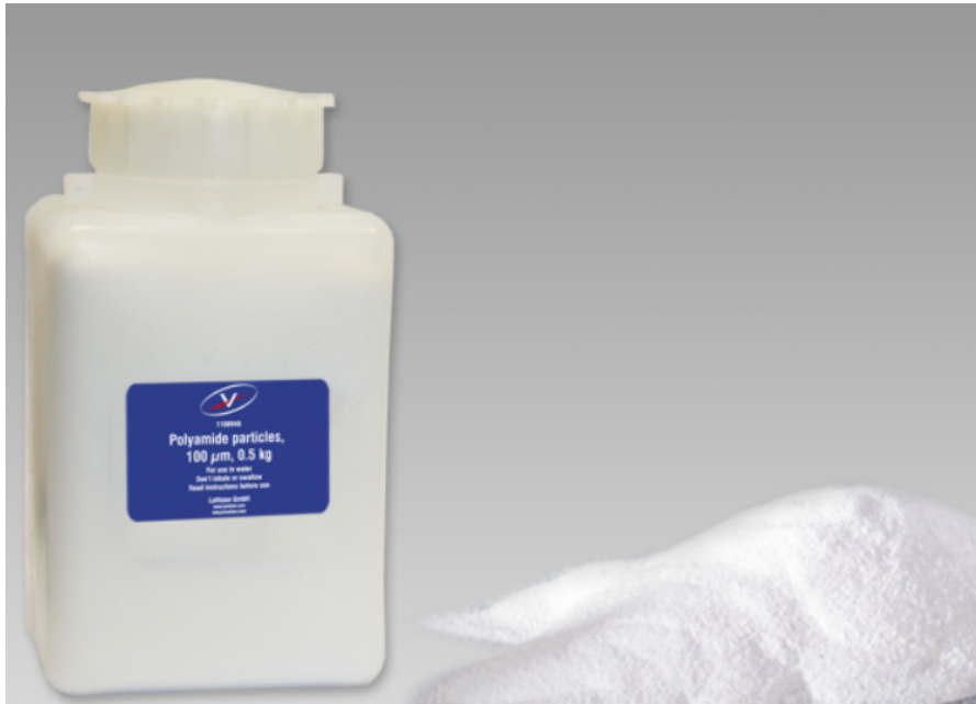
Figure 5.12: Particles used during the experimental tests d = 100 \mu m , \rho_p = 1100 \text{ kg/m}^3 [69].
