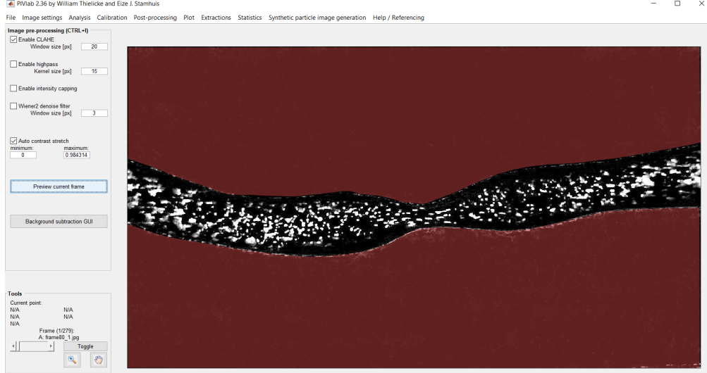
Figure 4.13: Example of applying the mask and Clahe filter to frames.
