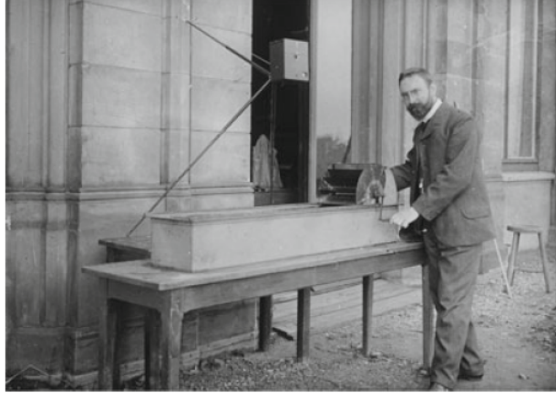
Figure 3.2: Ludwig Prandtl in front of his water channel for flow visualization in 1904 [32].
