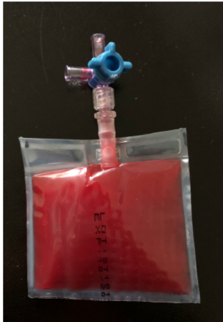
Figure 5.2: Bag made of PP with the liquid used as a dye inside [1].
