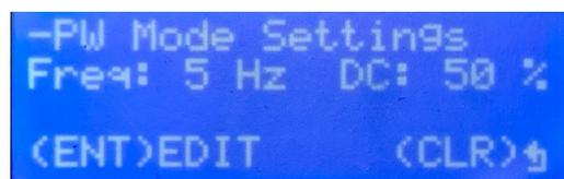
(f) Settings of frequency and duty-cycle in case of PW selection.
