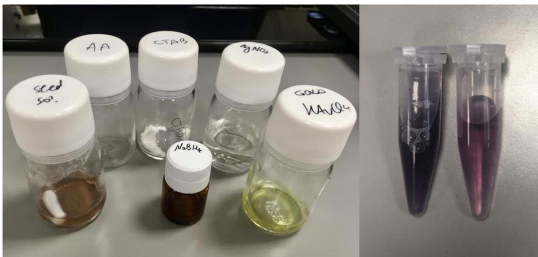
**Figure 13.** On the left side of the picture, we find all the materials diluted to obtain the desired concentrations and the brown seed solution; on the right the AuNRs solution before and after centrifugation steps.
