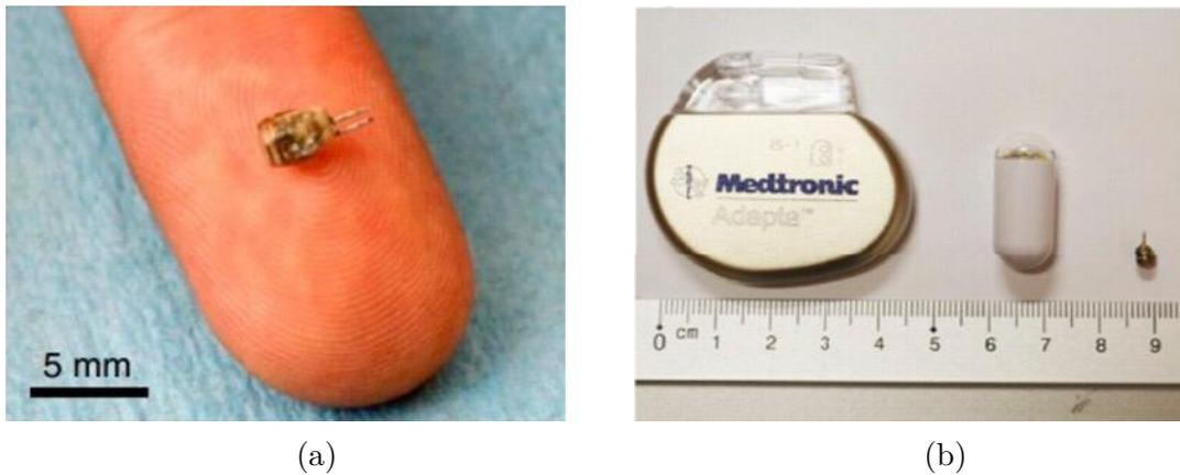
Figure 2.3: a) Electro stimulator miniaturized [4]. b) Battery-powered pacemaker (Left; Medtronic Adapta), battery-powered swallowable endoscope (Center), Electro stimulator (Right) [4].
