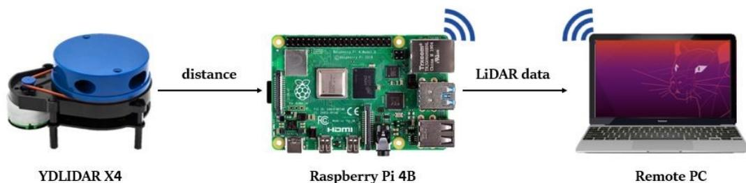
Figure 4.7: System setup for the implementation of the Hector-SLAM algorithm
