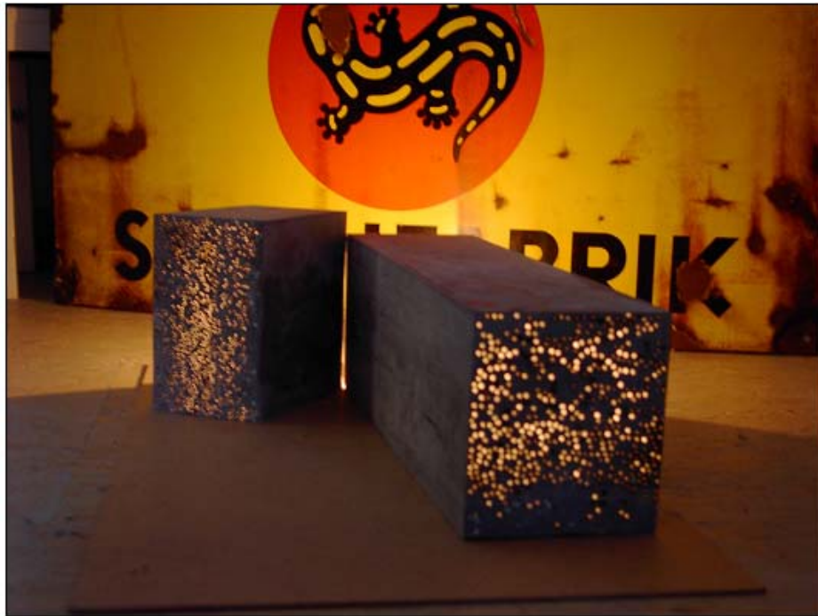
Transparent concrete blocks realized with optical fibres
