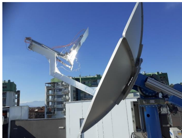
Figure 40 | Concentrator-receiver with the tracking system.
