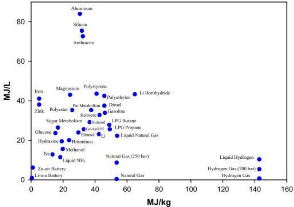
Figure 9: Volumetric vs Gravimetric energy density of a group of materials and technologies [33]
