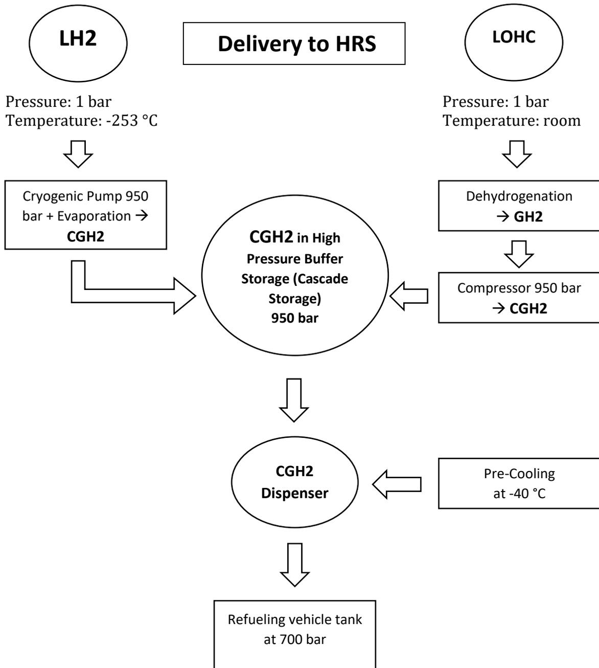
Depending on whether you arrive at the station LH2 or LOHC, you will have in the first case the structure of an LH2 Hydrogen Refueling Station (LH2 HRS), in the second one a LOHC Hydrogen Refueling Station. (LOHC HRS).
