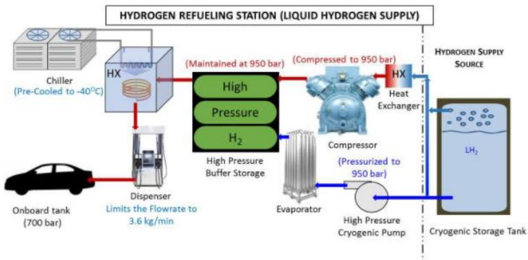
Figure 28: Configurations of LH<sub>2</sub> Hydrogen Refueling Station [57]
