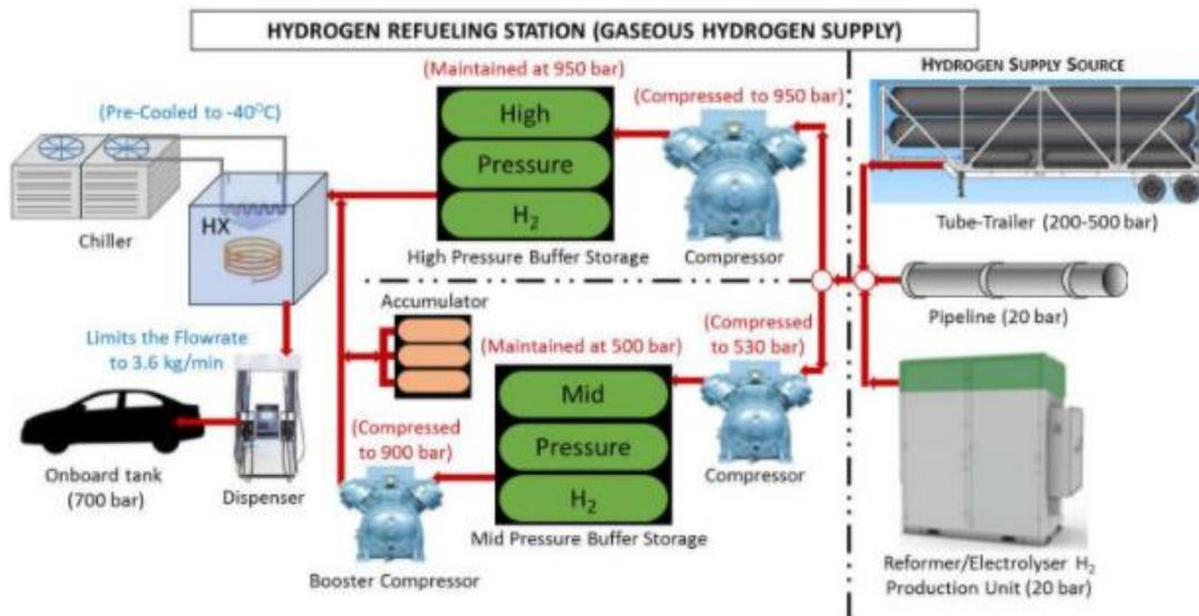
Figure 56: Configurations of CGH<sub>2</sub> Hydrogen Refueling Station [57]
