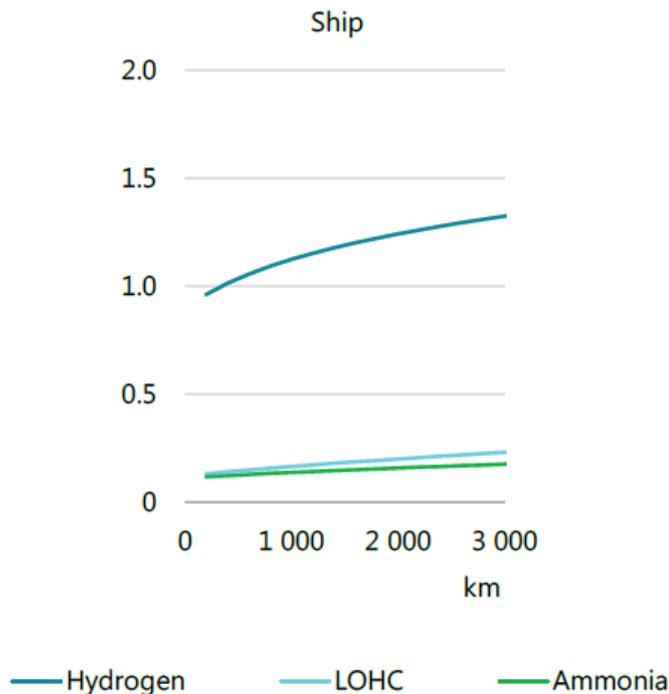
Figure 23: Cost of hydrogen transport by ship [5]
