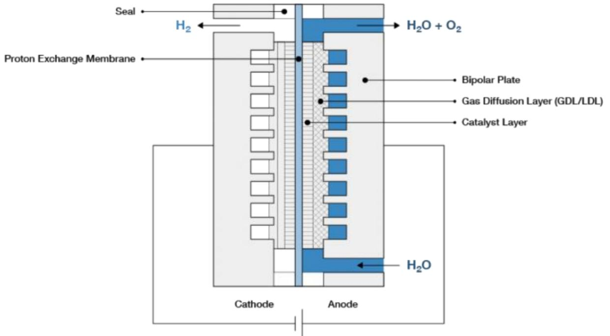
Figure 3: PEM Electrolyser Cell [20]
