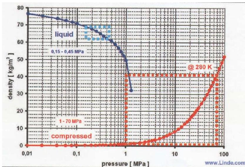
Figure 10: H<sub>2</sub> Density vs Pressure [34, from Linde.com]
