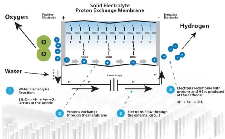
Figure 4: Solid Electrolyte Proton Exchange Membrane [21]
