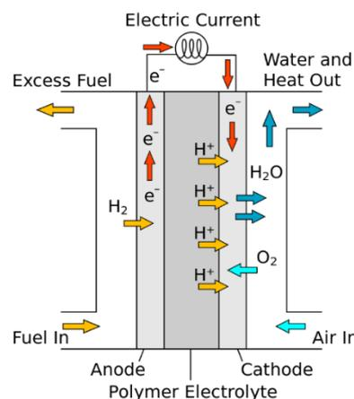
Figure 5: Diagram of a PEM Fuel Cell [27]
