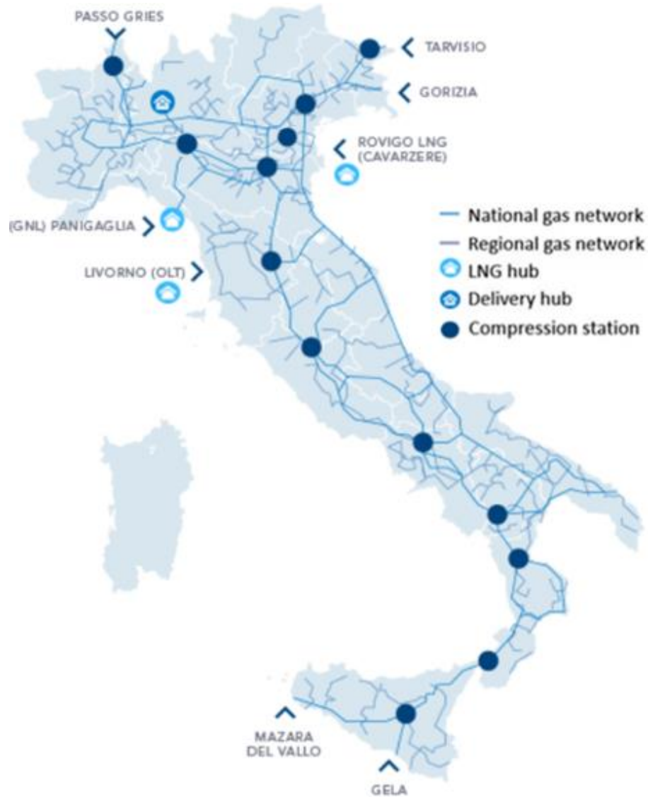
Fig. 1.18 The Italian natural gas pipelines network ( modified from [12] ).
