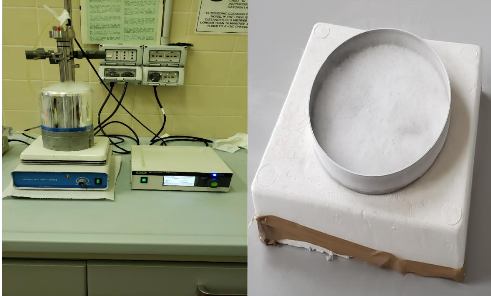
Figure 26. Spray-freezing system set-up (left) and collection tray (right)
