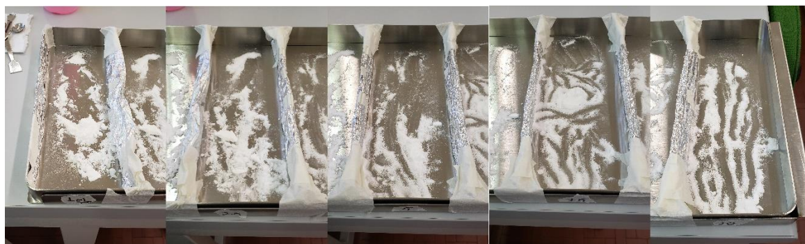
Figure 28. Tray containing the spray freeze-dried powder of the 40% (w/w) sucrose solution at different flow rates.
