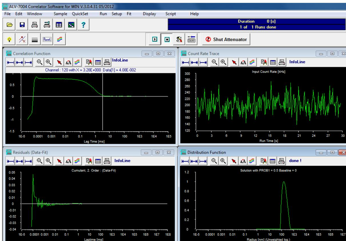
Figure 2.6: example of DLS measurement: on top left the correlation function curve, on top right the count rate trace, on bottom left the residuals and on bottom right the result of the distribution function, after fitting of the data.
