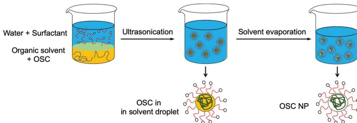
Figure 1.5: Elaboration of nanoparticles (NP) of organic semiconductors (OSC) via the miniemulsion process.<sup>5</sup>
