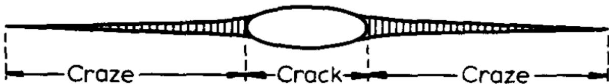
Fig.6 Schematic craze growth from crack tip
