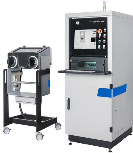
**Figure 24:** Mlab Cusing R L-PBF Printing Machine (*Concept Laser GmbH* (2021)).
