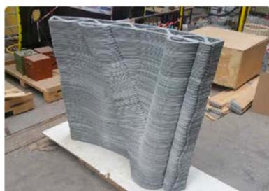
d) a vertically printed panel component: XTreeE, France
