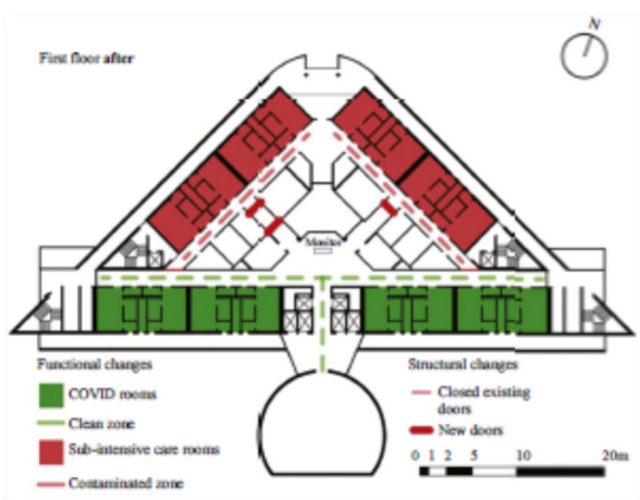
Picture 1. Plan of the first floor of San Matteo hospital after functional changes.
