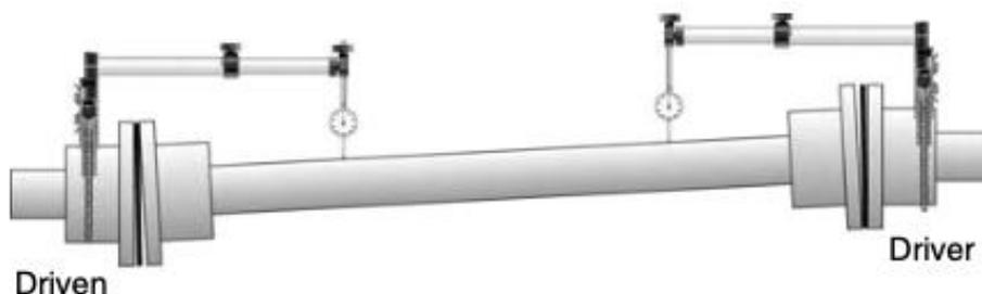
**Figura 2.19:** Shaft to coupling spool method
