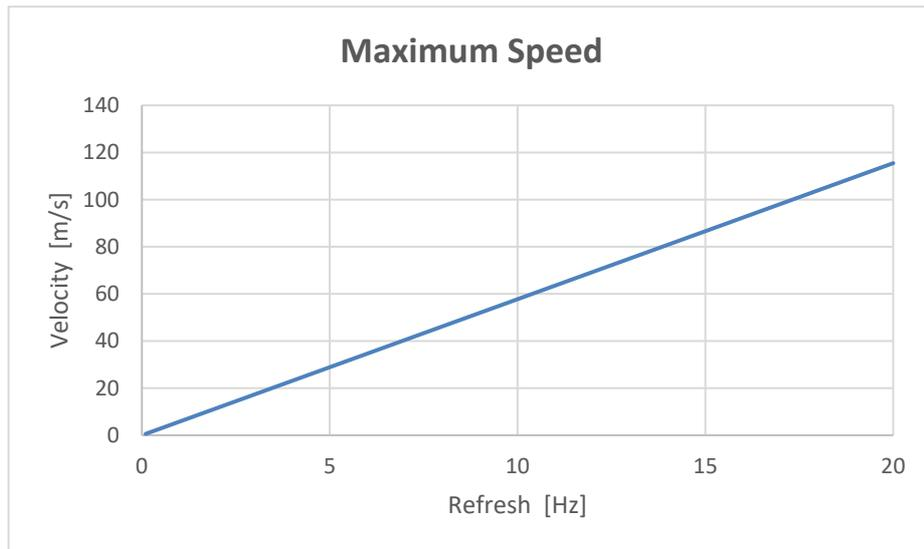
**Figure 40** Maximum speed according to the refresh rate with a distance from the walls set at 10m.
