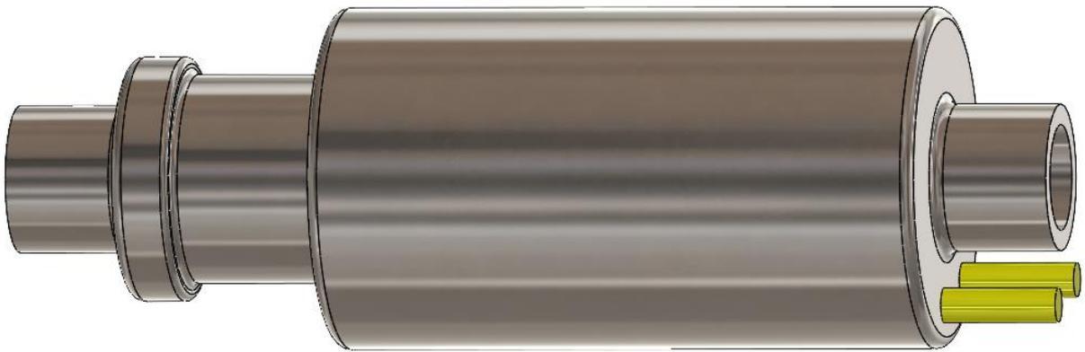
**Figure 77** Front view of a pintle [annex AD\_35]
