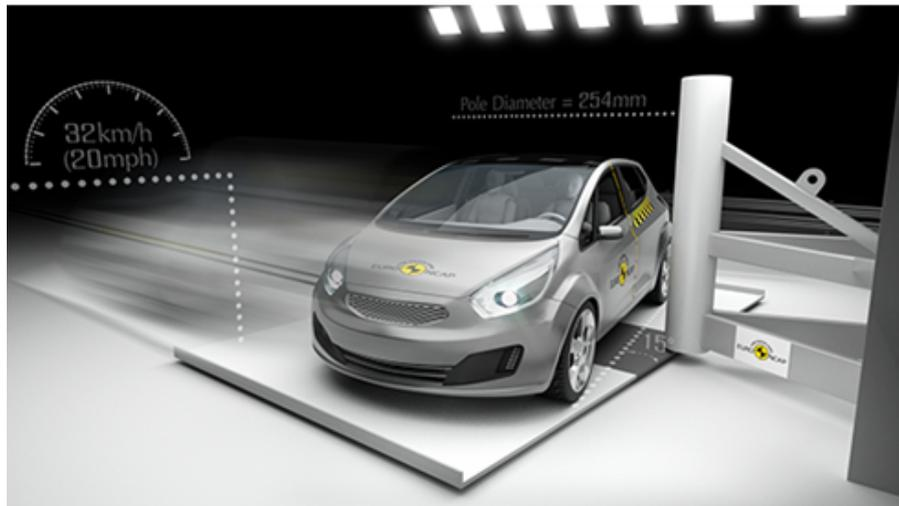
Figura 2.4: test side-pole Euro NCAP.
