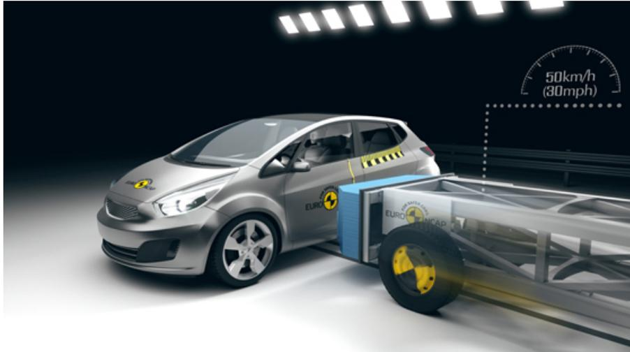
Figura 2.3: test Side impact Euro NCAP.
