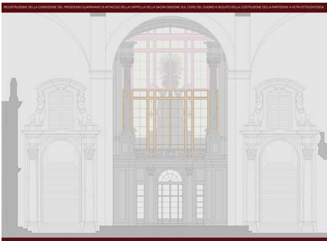
View Toward the Chapel of the Holy Shroud from the Nave of the Cathedral. Reconstruction of the front elevation of the 19th Century glass partition (original scale 1:50)
