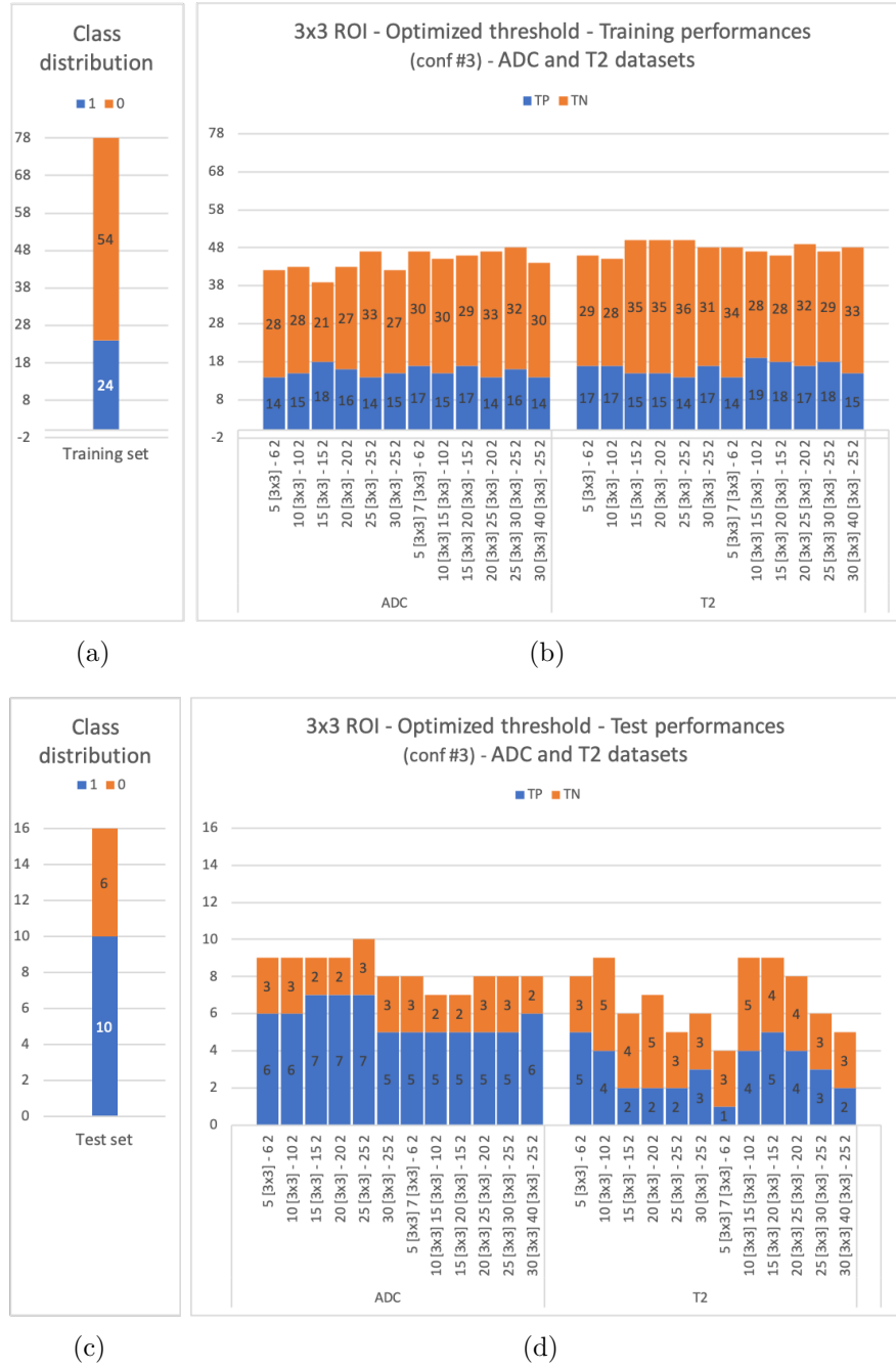
Figure 3.10: CNN results with training (b) and test (d) set, in terms of True Positive (TP) and True Negative (TN), for 3x3 ROI and lesion prediction #3, i.e. with optimized cut-off on ROIs and then on the MRI slices (see figure 3.7). (a) and (c) show the distribution of the two classes in training and test, respectively.
