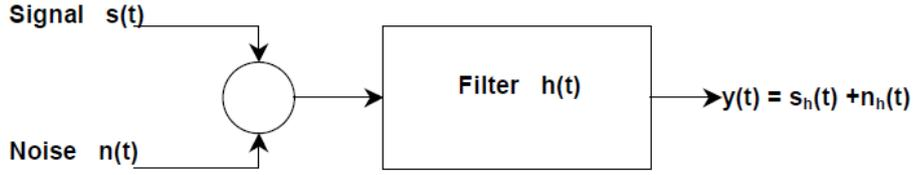
Figure 2.1: Basic filter structure
