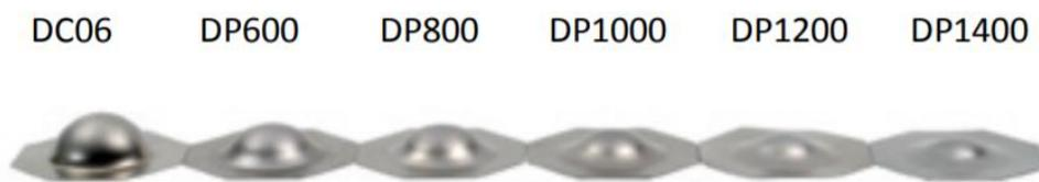
Figure 2.130 Drawing depth limits for several DP steels and a draw quality steel (DC)
