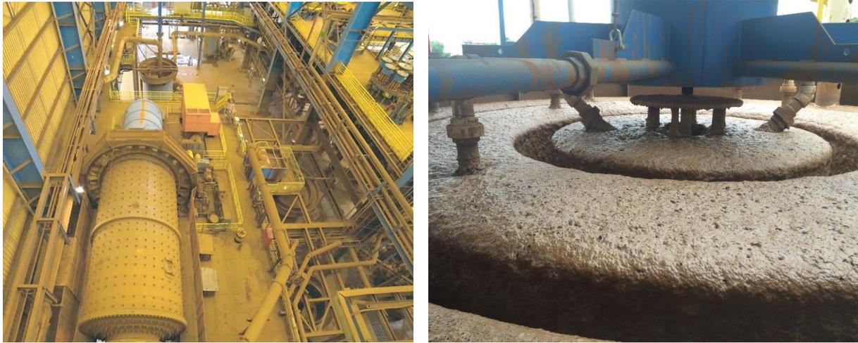
*Figure 1.4 (a) the crushing plant and (b) a flotation cell*
