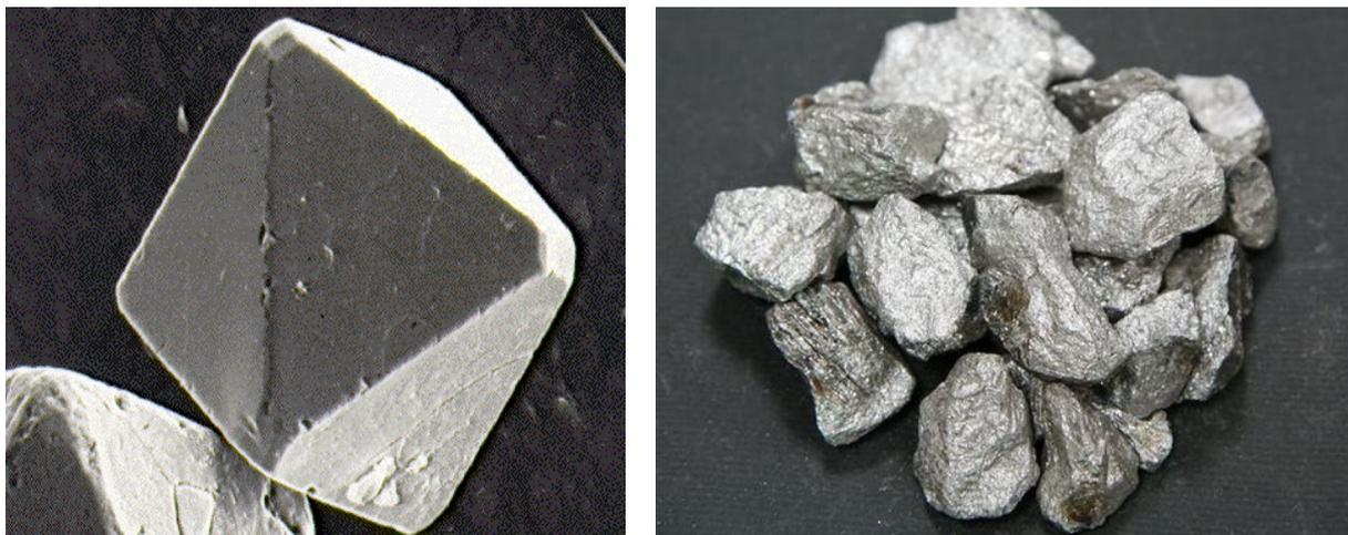
*Figure 1.3 (a) on the left a crystal of pyrochlore and (b) on the right the final product: ferroniobium*
